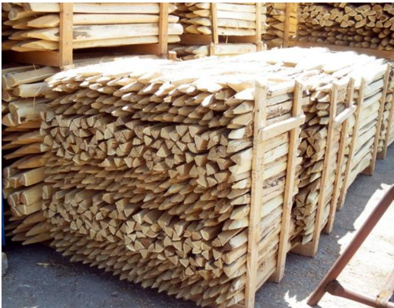
Figure 11 Squared posts from cleaven robinia wood stacked for shipment to customers. (Photo: FX Hardy OctoWood France, 2013)
