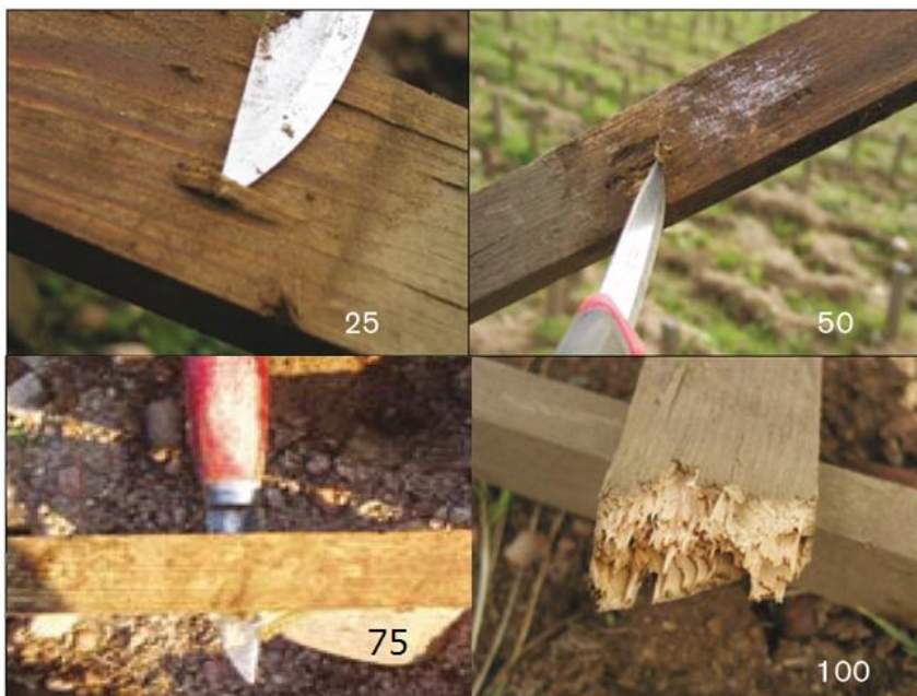
Figure 7 Rot index visualisation in compliance with the European field testing standard EN 252, used for analysing the degradation of timber in ground contact. (Reference: Råberg, Terziev 2006)
